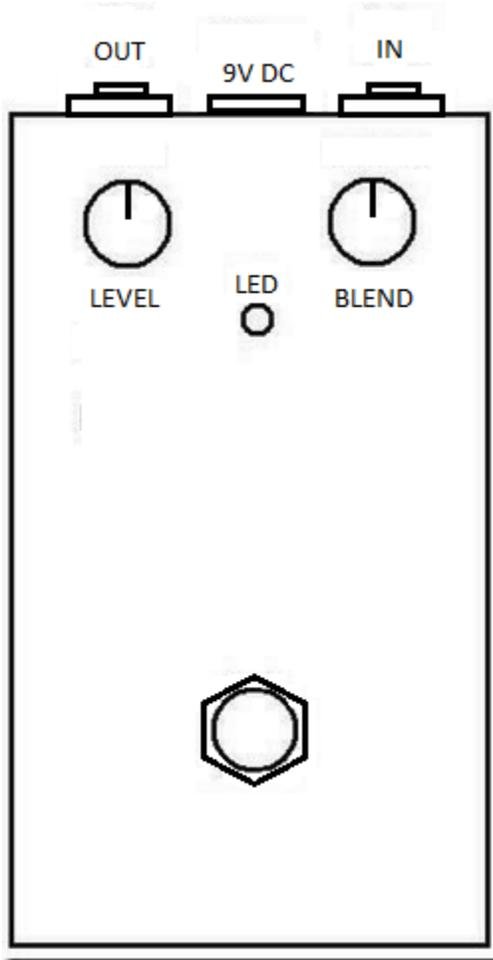
**Level:** Controls the overall volume of the pedal.
