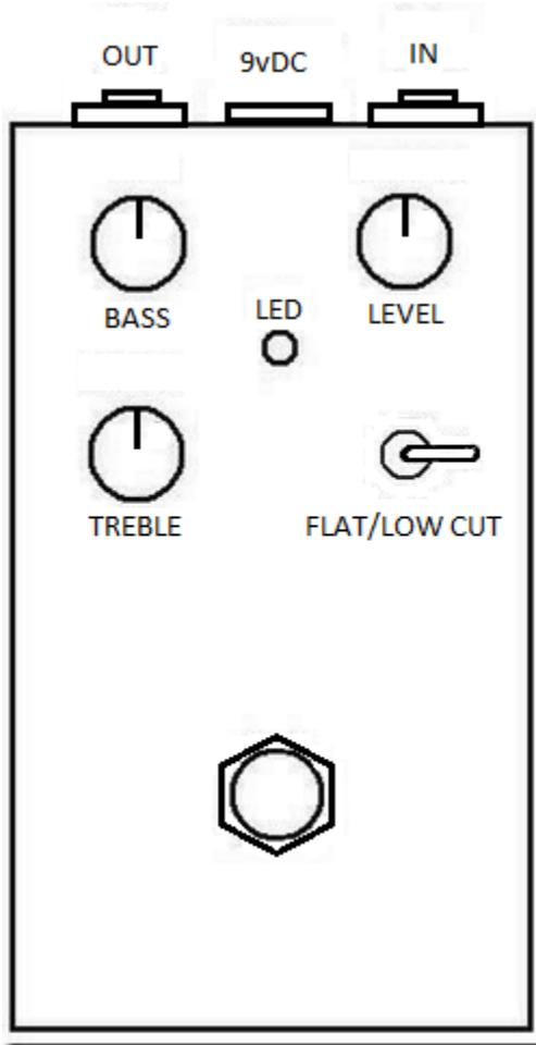
**Volume, Treble & Bass:** Fairly self-explanatory, however the Treble and Bass controls are a Baxandall type EQ which means that as the Bass and/or Treble controls are turned up the mid-range frequencies are decreased proportionally, conversely, when the Bass and/or Treble controls are turned down the mid-range frequencies are increased. Setting both controls at "noon" gives a fairly transparent EQ setting.
